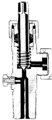
**Figure 2.3 Standard Cylinder Valve**
