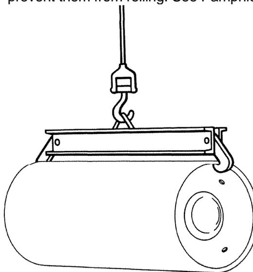
**Figure 2.6 Lifting Beam for Handling Chlorine Ton Containers**
